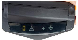
6.5 When about 5% of the battery capacity is left, the fan will begin to initiate an alarm and the battery symbol will flash. The battery capacity is sufficient to allow the work to be concluded without undue haste. The work should then be interrupted and the wearer of the equipment should leave the site
