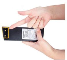
**2.1** Check before use that the gasket around the opening to the battery terminals are undamaged.
