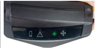
**6.3** After the internal test, all symbols will be extinguished except the small green fan symbol. This indicates normal operating status with a flow of at least 175 I / min.
