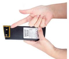
**1.3** Check that the gasket which is situated around the contact plate opening underneath the battery is intact.
