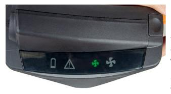
**10.3** If the flow meter outlet is now unblocked and the air is allowed to flow freely, the alarm signals will cease within 10 – 15 seconds.
