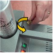
For maximum smoke output adjust flow control **fully anticlockwise**.
