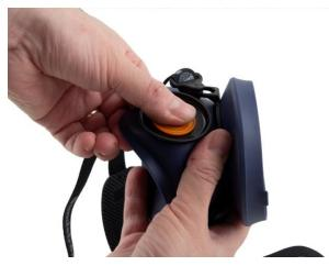
**7.3** Press the new membranes onto the dowels. Carefully check that the membranes are in contact with the membrane seats all round.
