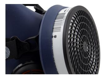
**1.5** Fit the filter/combined filter in the mask so that the arrows on the filter point towards the user's face. Carefully check that the edge of the filter is in the internal groove of the filter mounting all around.
